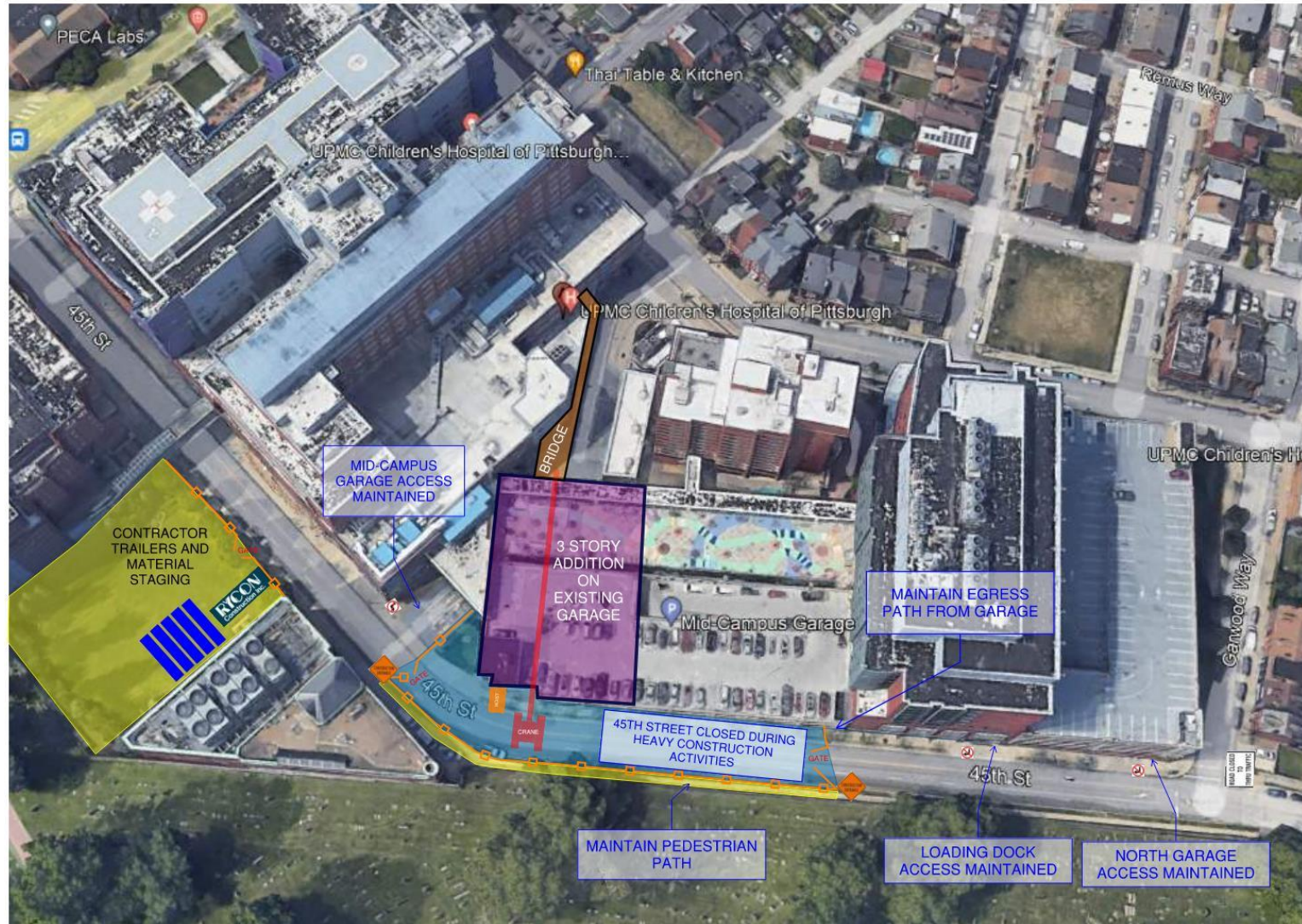
Phase 2 Includes Sidewalk and Full Lane Closures Duration Approximately 10-12 Months
